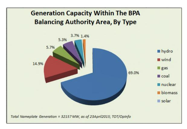
On the other hand, wind's "nameplate capacity" is 14.9% of the 32,157 MW, or 4,791 MW. The BPA wind nameplate capacity is slightly more than four times the nameplate capacity of CGS.
