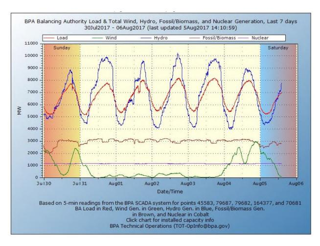
Nuclear is the almost horizontal blue line on the BPA Generation plot at about 1,200 MW. Note that the total generation is in excess of "BA load" as the BPA exports surplus power to locations such as southern California via the Pacific Intertie.
