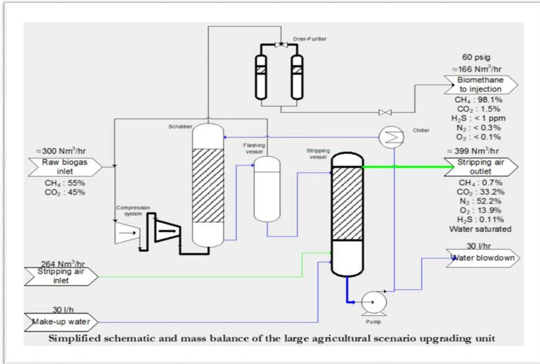
Figure 19. Upgrading schematic for dairy biogas from Electrigaz (2011).
