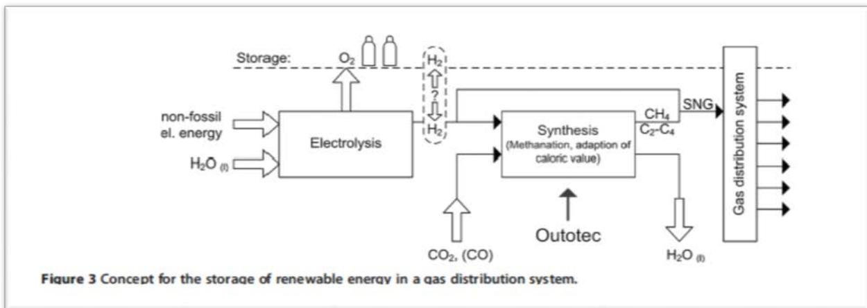
Figure 32. Methanation Concept for producing renewable methane from electrolytic hydrogen and CO<sub>2</sub><sup>92</sup>.
