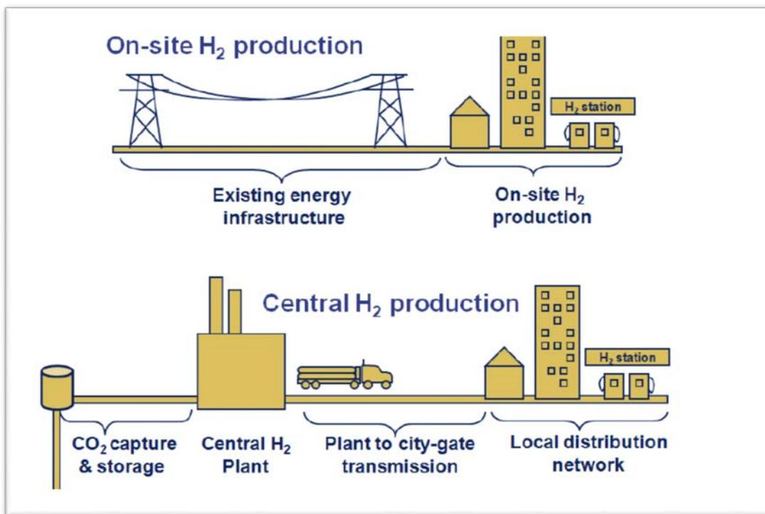
Figure 14. Centralized and onsite hydrogen infrastructure pathways for providing hydrogen transportation fuel.<sup>77</sup>
