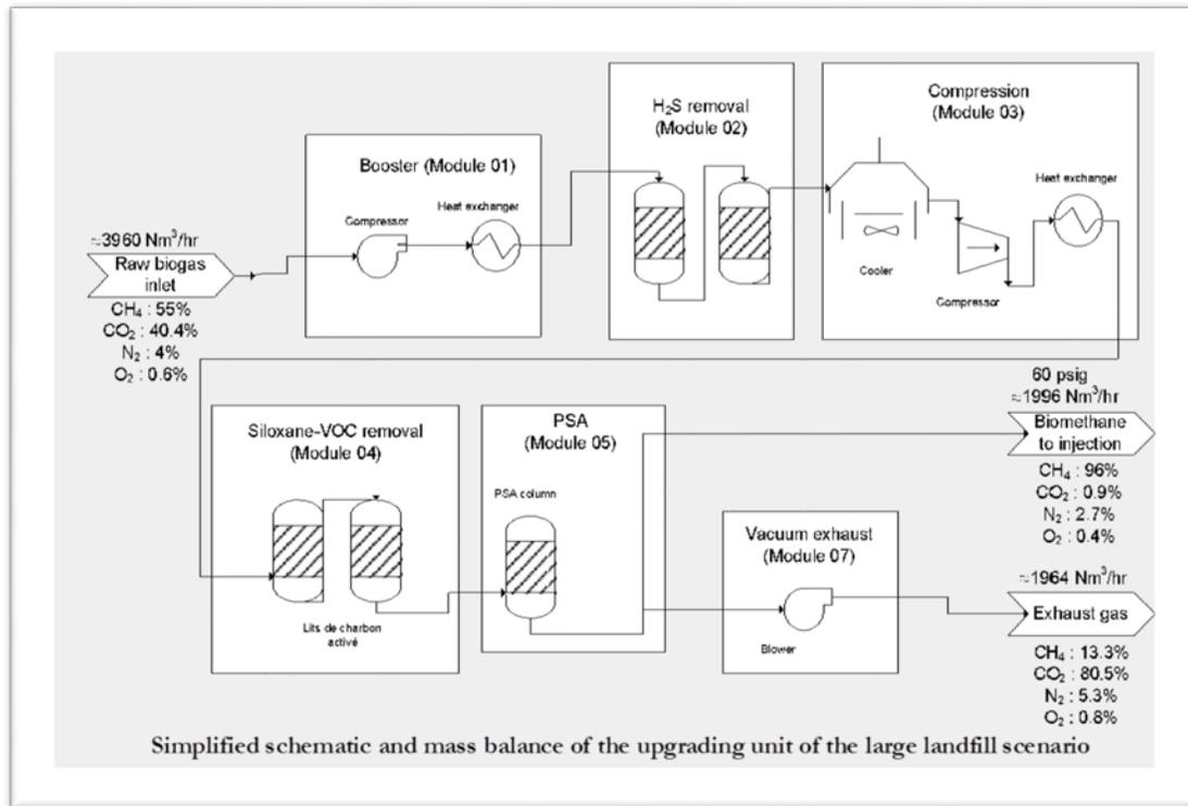
Figure 20. Upgrading schematic from LFG from Electricgaz (2011).
