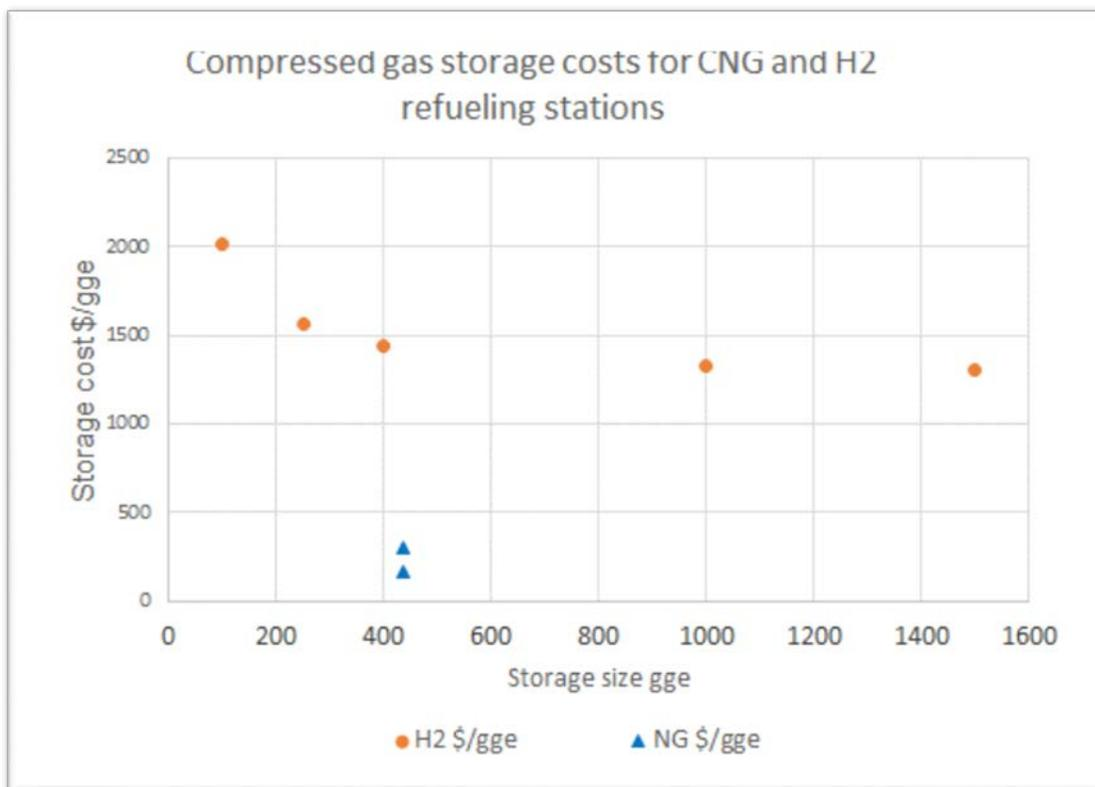
Figure 27. Cost comparison for H<sub>2</sub> and CNG refueling station compressed gas storage tanks versus tank size. The H<sub>2</sub> tank is 425 bar pressure and the CNG tank 245 bar.
