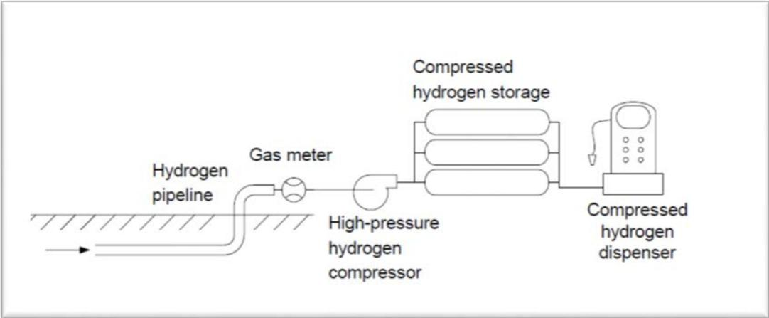
Figure 16e. Hydrogen station with hydrogen pipeline delivery.
