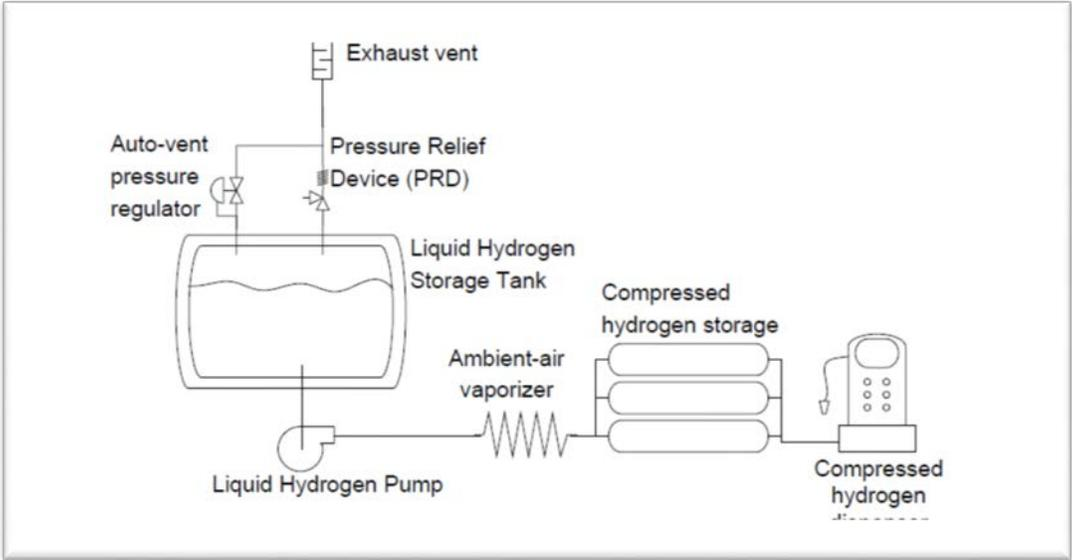
Figure 16d. Hydrogen station with liquid hydrogen delivery.
