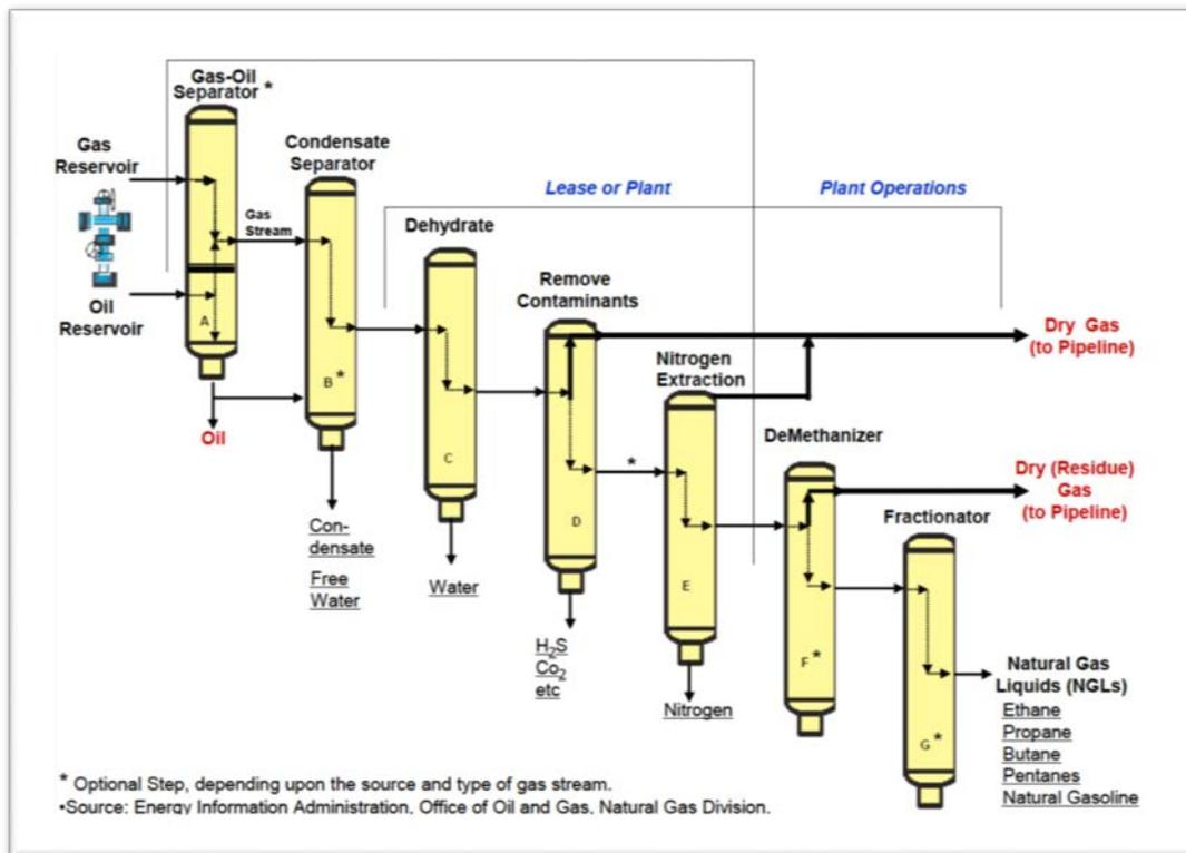
Figure 18. Generalized Natural Gas Processing Schematic from Electrigaz (2011).
