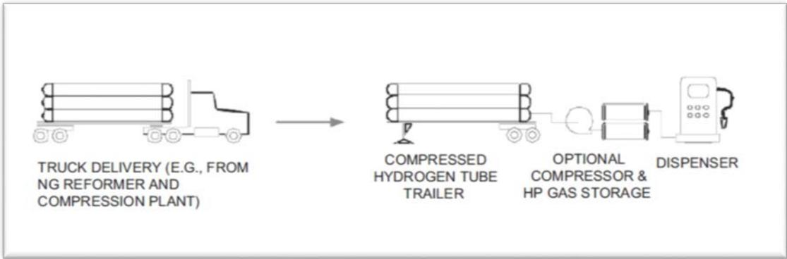
Figure 16c. Hydrogen station with compressed gas truck delivery
