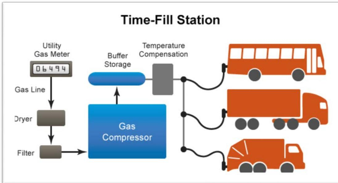
Figure 11. CNG Time fill station configuration.
