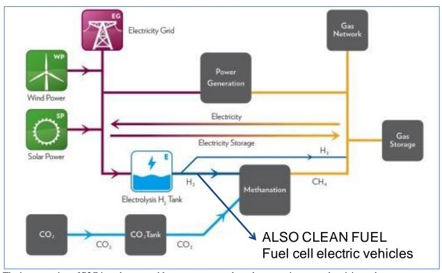
The incorporation of P2G into the renewable energy system, the only way to integrate electricity and gas sectors
