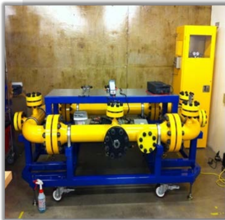
Natural gas pipeline sensors testbed at UC Berkeley
