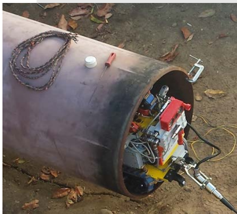
Diakont's Robotic Operational Defect Inspection System (RODIS) at the pipeline entry
