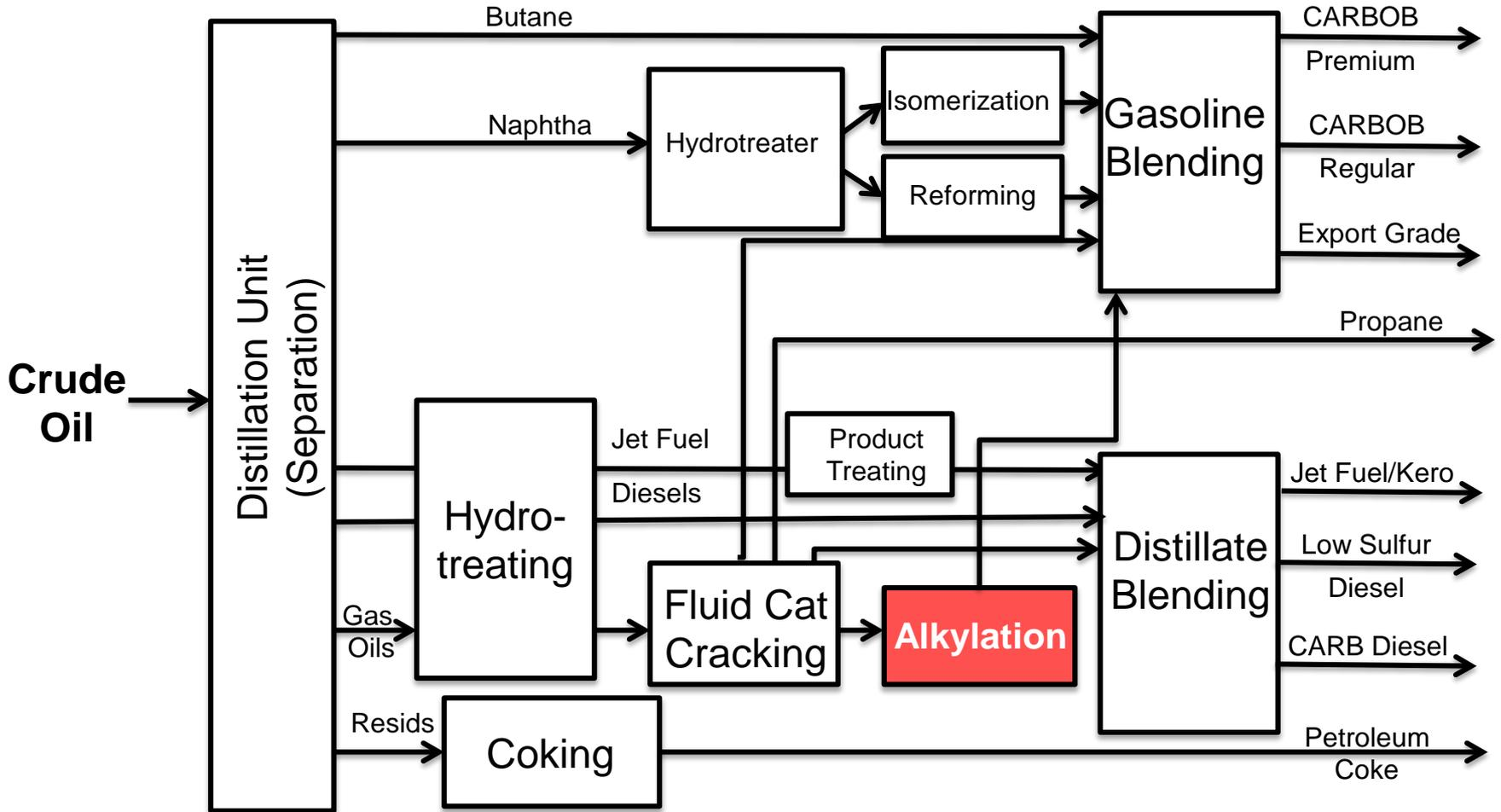
*Then the refinery upgrades, cracks, and recombines the molecules*
