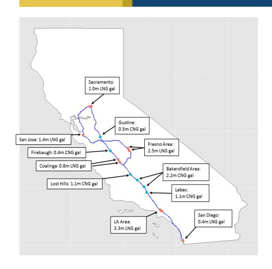
Initial locations of LNG (red dots) and CNG (blue dots) refueling infrastructure and route deployment.
