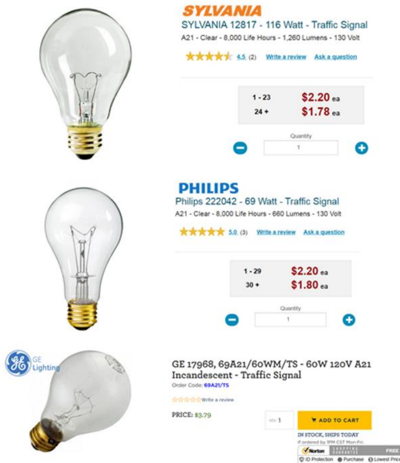
Figure 4.7 – Examples of traffic signal lamps available from 1000bulbs.com 24 and topbulb.com 25 look like typical A-shape, E-26 medium base incandescent lamps
