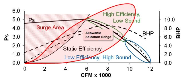
The FEI metric will reinforce positive market behavior by design engineers, contractors and manufacturers. The performance bubble will encourage design engineers and contractors to optimize system design and fan installation to assure fans perform within the allowed operating range. Fan manufacturers will strive to develop fans with a large performance bubble to meet the requirements of design engineers and installing contractors.
