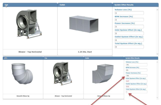
In this example, adding an elbow to the inlet of the fan and replacing the straight duct on the discharge of the fan with an elbow increases the Pressure Drop (i.e. Total System Effect) by 1 in. wg. and the fan power consumption by 18%. (ref. Greenheck System Effect Simulator - https://ses.greenheck.com/)
