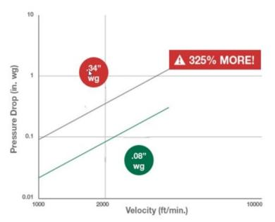
It is intuitive that a damper with 325% more pressure drop will result in a significant increase in fan power consumption. Failure to accurately account for the pressure drop of specific components, such as dampers, will be compensated for in the fan selection. The result will be a fan that is under-optimized for the application and will likely require significantly more power consumption than necessary to meet the airflow requirements of the system.
