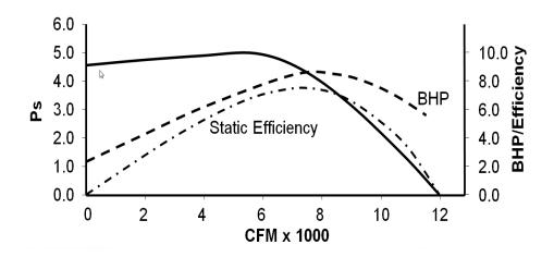
This curve shows that the Static Efficiency for a fan can vary from 0% to a peak efficiency of around 80% (peak efficiency will vary by fan type). Depending on the application requirements of a fan (e.g. flow, pressure, space constraints, sound, etc.) focusing on only peak efficiency can be misleading and will not always result in the use of a fan that minimizes energy consumption.
