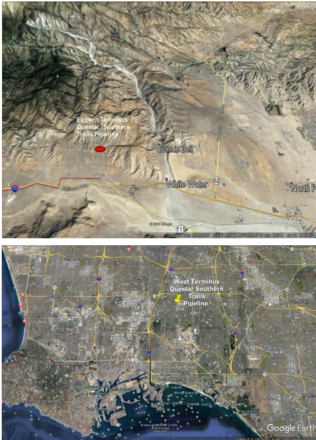
Figure 12. Western Section, Southern Trails Pipeline, east and west terminals. This pipeline is for sale by Questar. Former crude oil pipeline, now out of service: 16" diameter, 96 miles long, without compression or other midline components. It might be repurposed for low-pressure, low-capacity, gaseous Hydrogen (GH 2 ) service as a "lighthouse" project, in the short term. If relined to 12" diameter, MAOP = 100 bar, pipeline capacity would be ~ 900 MW = ~ 400 metric tons (Mt) of Hydrogen fuel per day = 40,000 kg / day. Contact: Lori.Creer@questar.com
