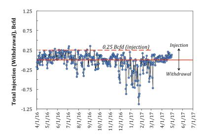
Figure 2 – Total Gas Injection and Withdrawal from the three Currently Operated Storage Fields since April 1, 2016
