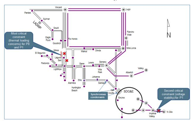
Figure 6.3-4: Transmission constraint identified for the LA Basin and San Diego areas (with peak shift modeled for the study)
