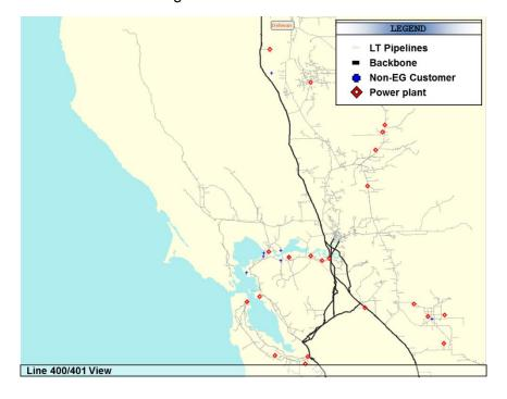
The aggregated capacity of power plants served from Kern River-Mojave gas system is roughly 3,800 MW of which 2,200 MW is in PG&E service territory and 1,600 MW is in SCE territory.
