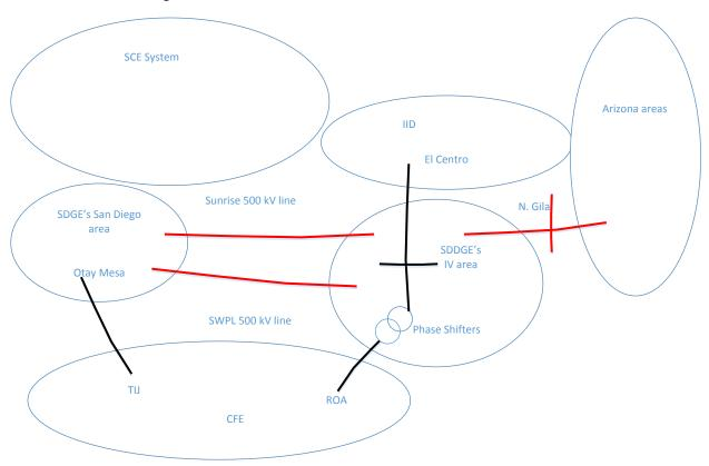
Figure 4.7-4: SDGE/IID/CFE area electrical interconnections
