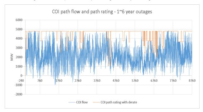
Figure 4.7-3: COI path flow and path rating with 1~6 year outages modeled
