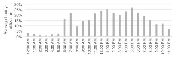
Figure 2: Hourly utilization rates of an individual EVgo host site
