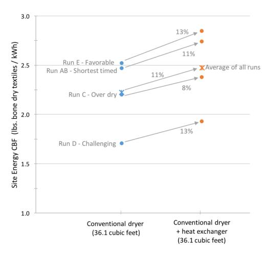
Figure 6.3 Test results of commercial tumble dryer with heat exchanger installed
