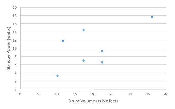
Figure 4.1 Standby power of seven commercial tumble dryers
