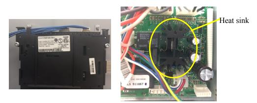
Figure 6.7 Control circuits for vended Dryer 6 (left) with 3.3 W standby power and vended Dryer 5 (right) with 14.5 W standby power
