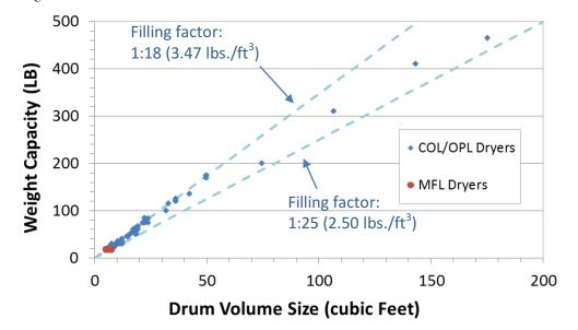
Figure 3.6 Relationship between drum volume (cubic feet) and load weight capacity in commercial dryer specification sheets (up to 200 cubic feet)
