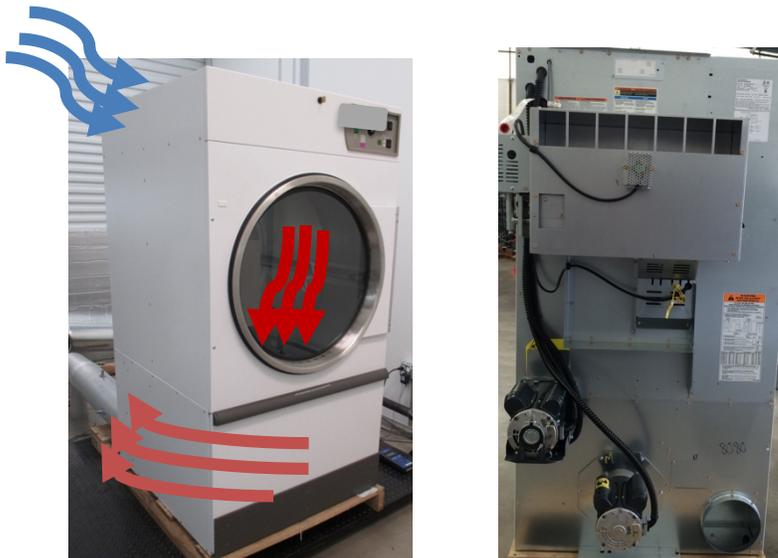
**Figure 3.1 Airflow through a commercial tumble dryer (left) and photo of rear of tumble dryer (right)**
