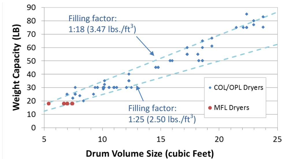
Figure 3.7 Relationship between drum volume (cubic feet) and load weight capacity in commercial dryer specification sheets (up to 25 cubic feet)
