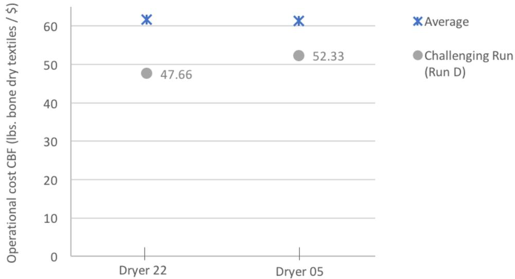
**Figure 5.5 Difference between Average CBF and CBF of Run D for dryers tested by the CASE Team**
