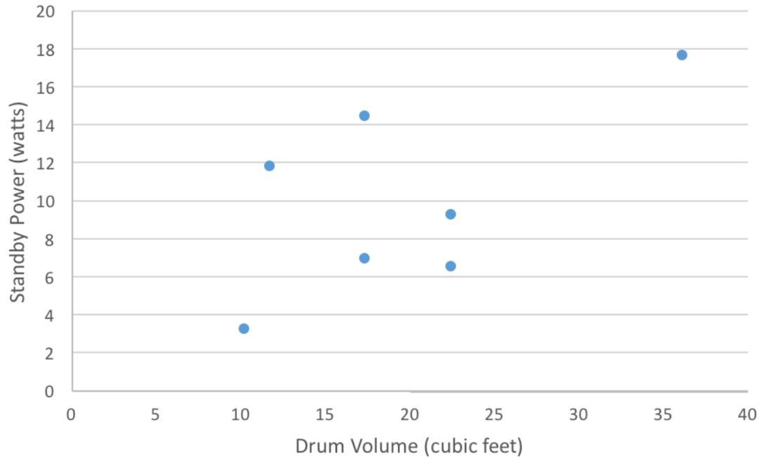
**Figure 4.1 Standby power of seven commercial tumble dryers**
