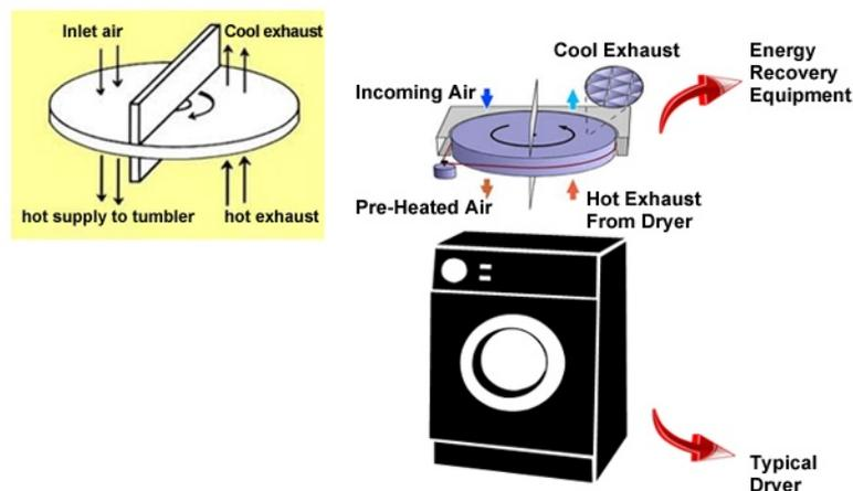
**Figure 6.1** How a heat exchanger works with a dryer
