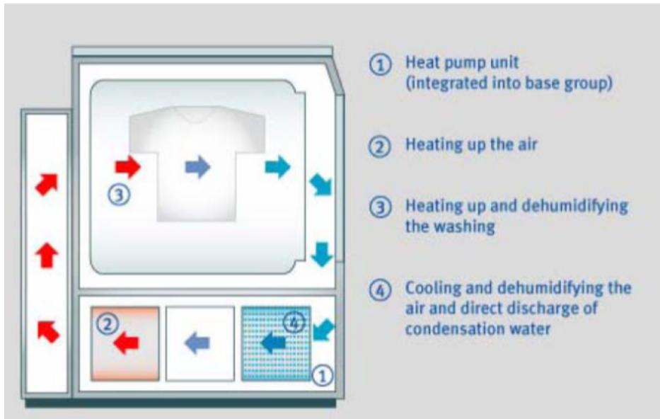
**Figure 6.6 How an electric heat pump dryer works**
