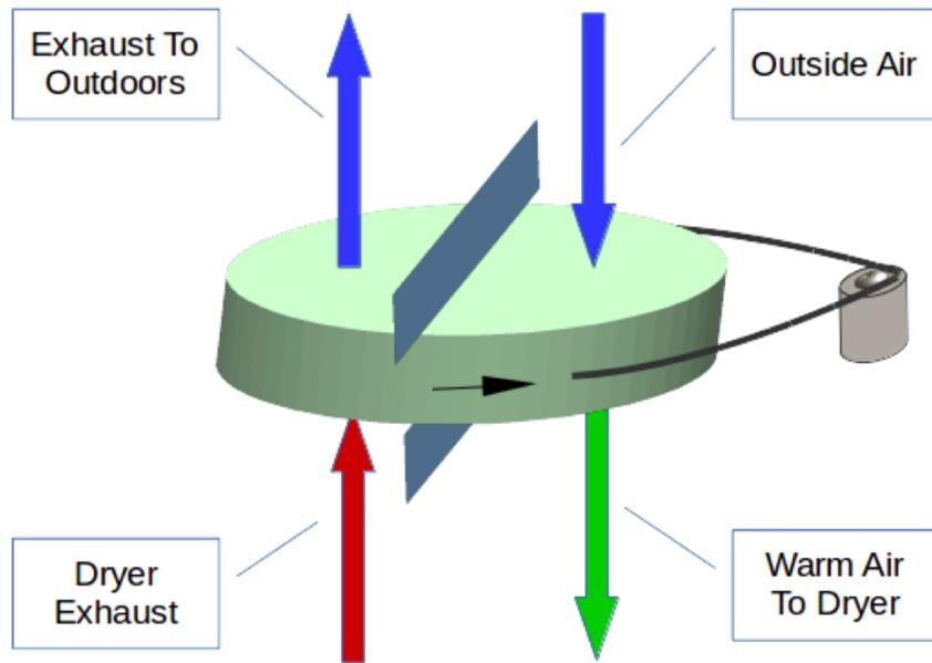
**Figure 6.4 Heat recovery wheel with self-cleaning reversing airflow**
