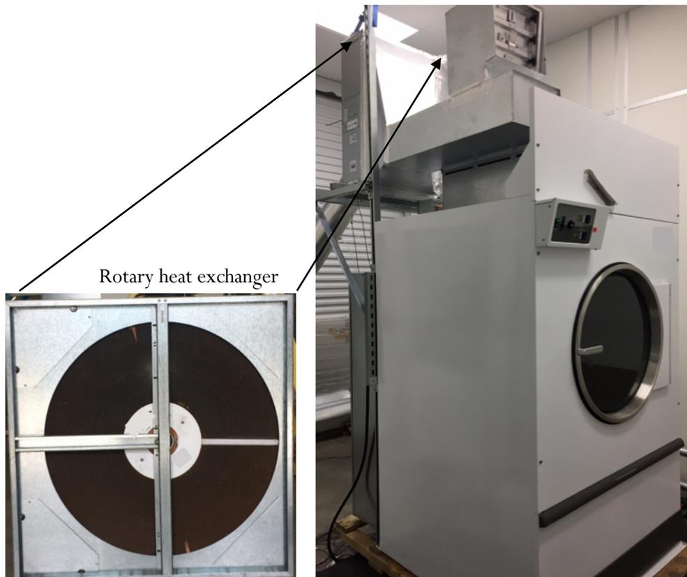
**Figure 6.2 Rotary heat exchanger before installation on dryer (left); dryer with retrofitted heat exchanger in test chamber (right)**
