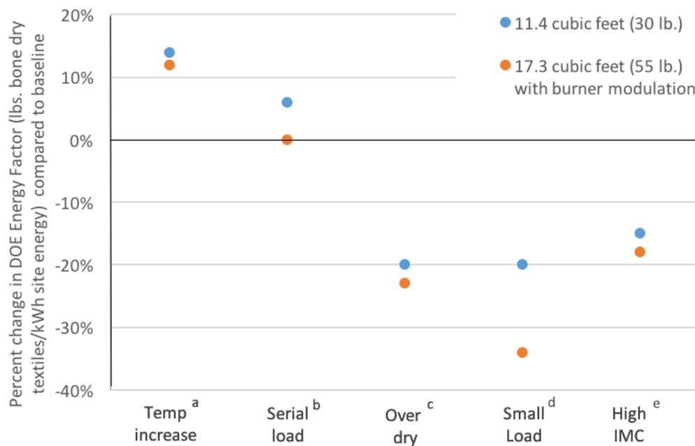
**Figure 5.1 Efficiency impact associated with isolated variable change for two dryers (11.4 and 17.3 cubic feet).**
