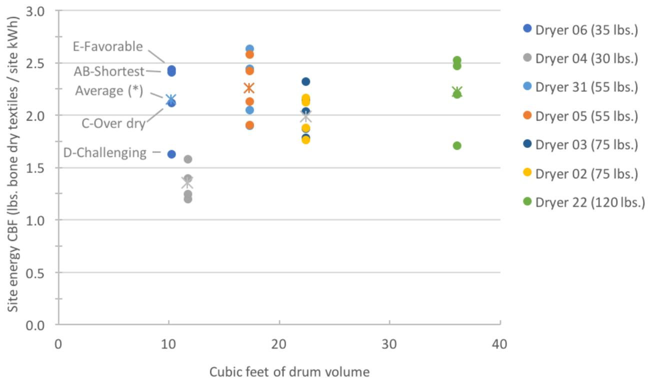
**Figure 5.4 Summary of CASE Team measurements of commercial dryer energy efficiency**
