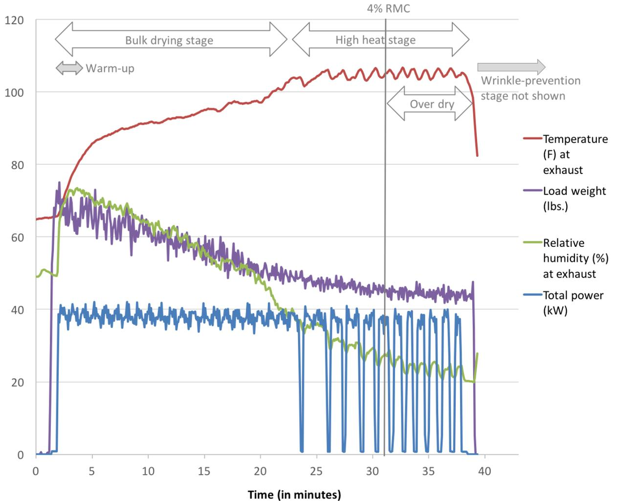
**Figure 3.5 Typical drying cycle for commercial tumble dryer (shown: 17.3 cubic foot, 55 pound capacity dryer)**
