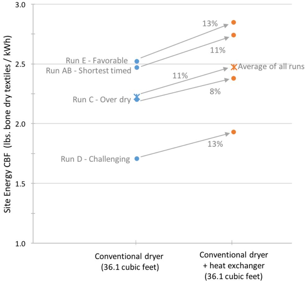
**Figure 6.3 Test results of commercial tumble dryer with heat exchanger installed**
