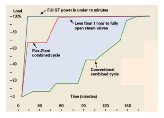
**El Segundo performance.** Each 5000F 1x1 Flex-Plant 10 is design rated (at 85°F) to deliver 150MW of gas turbine power in 10 minutes (non-spinning reserve) for peak backup of intermittent renewable generation and full 275MW plant output at 48.8% efficiency in less than 60 minutes.
