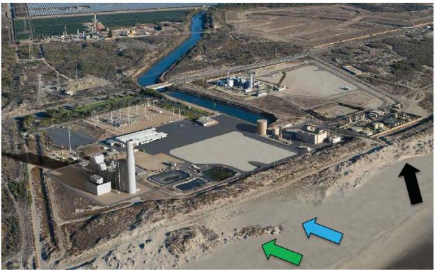
Figure 2. Photo from FSA showing view of Puente site with an artistic rendering to show a potential post-construction removal of the existing outfall structure. The black arrow indicates recent dune erosion and the blue arrow shows area of recent wave overtopping to the access road. The green arrow shows part of the area of substantial dune erosion depicted Figure 3.
