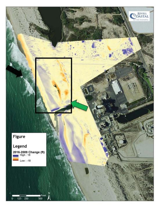
Figure 3. Topographic changes between 2016 and the 2009 LIDAR. The hot colors indicate erosion and the cool colors indicate accretion. The black arrow is the approximate view angle for the FSA cover image and the black box highlights the area of greatest change in front of the proposed Puente project. The green arrow approximates the dune identified with the same arrow in Figure 2.
