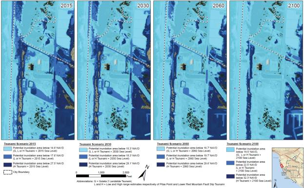
Potential Tsunami Inundation Mapping in the Vicinity of Mandalay Bay Generating Station
