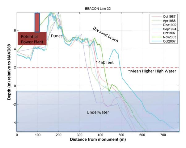
Figure 5. Beach showing elevations and topography through time collected from just north of the
