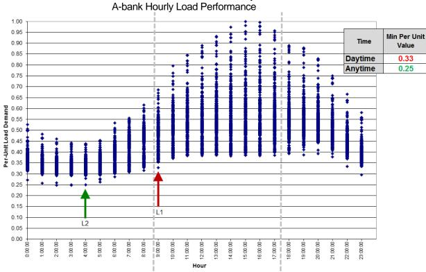
Figure 3.2.2 Normalized Local Subtransmission System A-bank Hourly Load Performance
