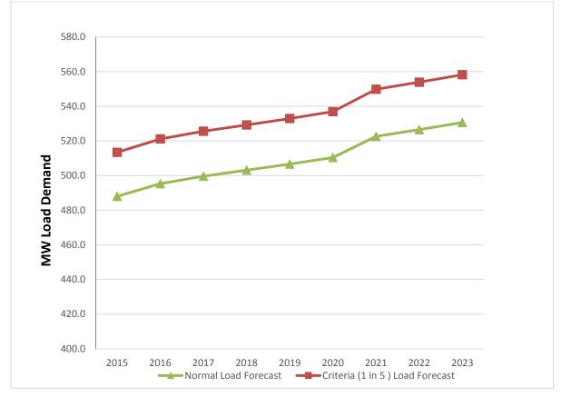
Figure 3.2.1 Barre AB A-bank Load Forecast
