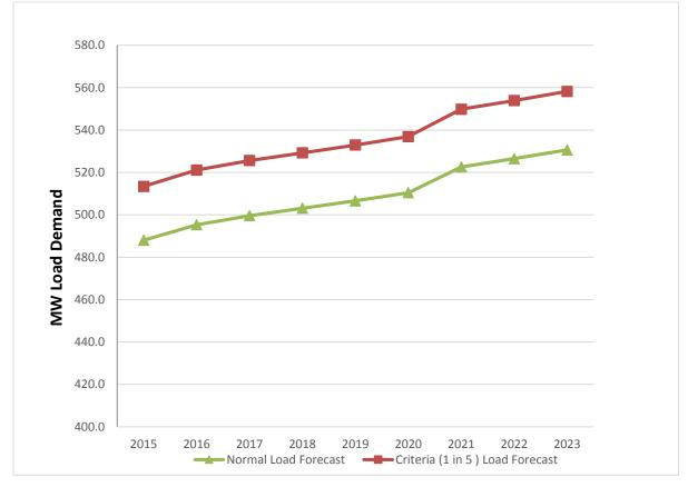
Figure 3.2.1 Barre AB A-bank Load Forecast
