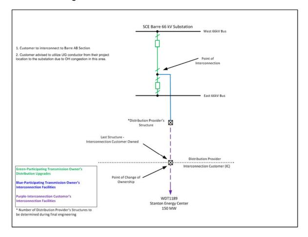
7. One-Line Diagram of Interconnection to Barre 66 kV Substation.
