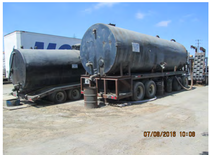
18. View of the oil truck parking area in the central/western portion of the Site with draining to open drums and containers visible.
