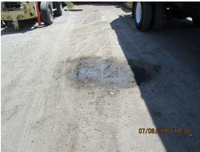
19. View of oil-stained soil in the un-paved truck parking area in the eastern area of the western portion of the Site.
