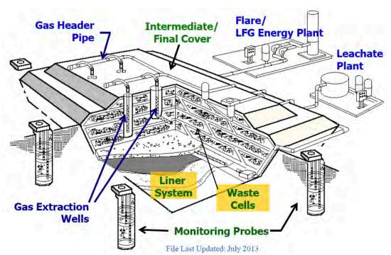
Figure 1 Biogas Formation and Treatment Steps at Municipal Sanitary Landfills
