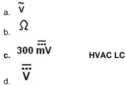
A normal thermocouple out-put is 30 mV DC. The correct setting would be 300mV DC.
