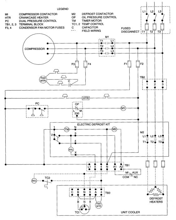
134. The compressor on a walk-in freezer has just restarted after a defrost cycle but the technician notices that the evaporator fans are not operating. What would the first component that the technician would focus on in this situation?
