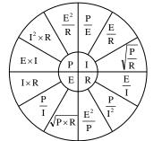
E = voltage I = current (amps) P = power (watts) R = resistance (ohms) W = energy (kWh, or kilowatt-hour) t = time (hours) **Sum of resistance** *Series circuits*
