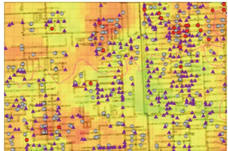
Figure 1: Predictive Heat map shows data sources indicated by symbols below, which illustrates, i.e. historical leaks, customer calls, and condition-assessment data clustering.
