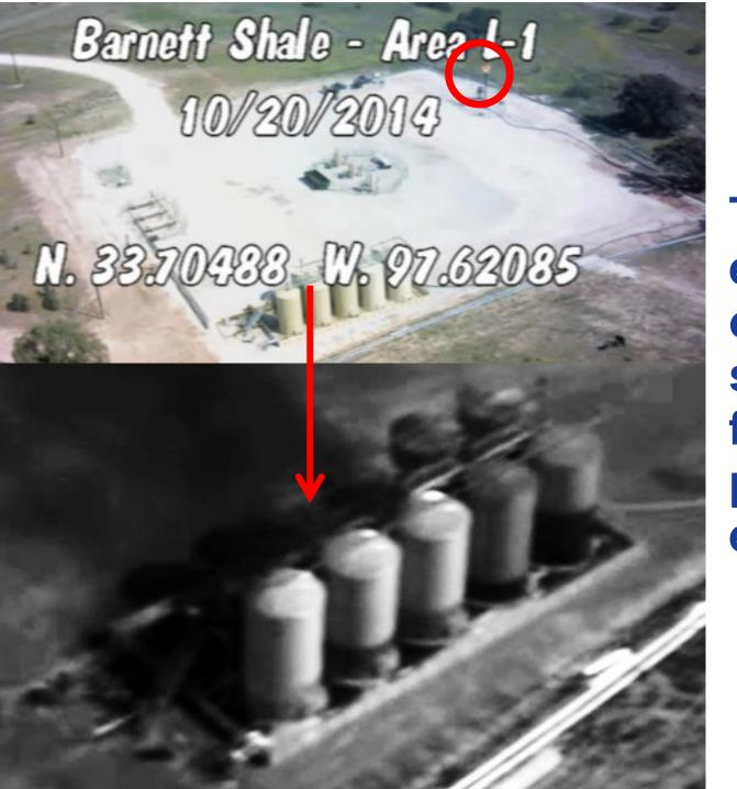
Tank hatch emissions observed at sites with flares indicate poor capture efficiency.
