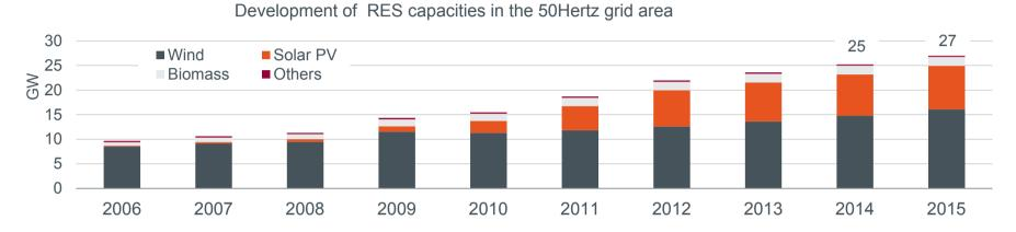
Development of RES feed-in (according to EEG) in the 50 Hertz grid area TWh
