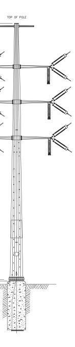
Double Circuit Dead End Structure Type C
