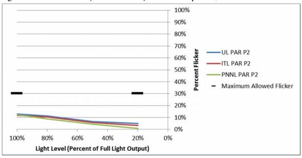
Figure 19: Flicker test data (filtered <200 Hz) three lab comparison, PAR P2<sup>15</sup>
