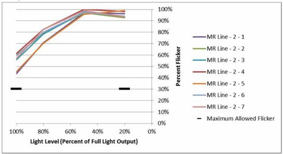
Figure 2: Percent Flicker (Filtered <200 Hz) vs. dimming level for MR Line 2, all 7 configurations
