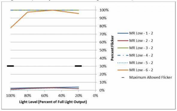
Figure 6: Percent Flicker (Filtered <200 Hz) vs. dimming level for all MR Low Voltage lamps, configuration 2 (forward phase cut dimmer and magnetic transformer)
