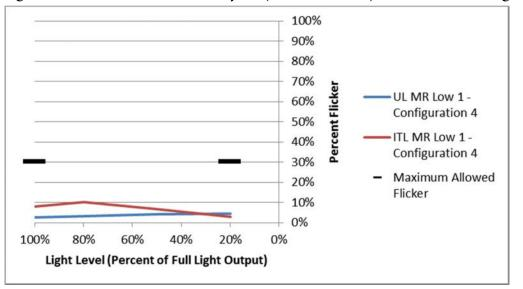
Figure 18: Round robin test results by lab (filtered <200 Hz) for MR Low 1, configuration 4
