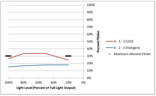
Note that in Figure 2 the LED A-Type lamp exceeds 30 Percent Flicker at 50% and 80% of rated light output. But because measured flicker at 20% and 100% full light output is less than 30 percent flicker, the lamp complies with the California flicker requirements.
