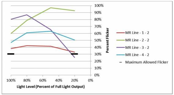
Figure 5: Percent Flicker (Filtered <200 Hz) vs. dimming level for all MR Line Voltage lamps, configuration 2
