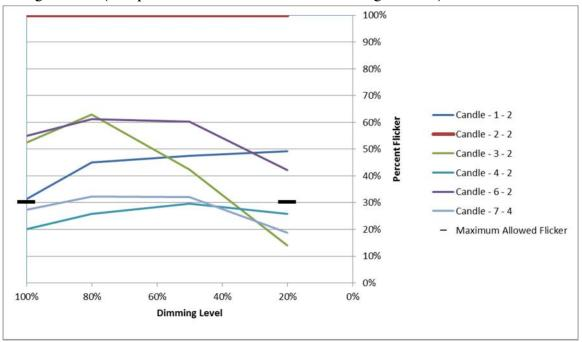
Figure 7: Percent Flicker (Filtered <200 Hz) vs. dimming level for all Candle lamps, configuration 2 (Except for Candle – Phase 3, tested in configuration 4)
