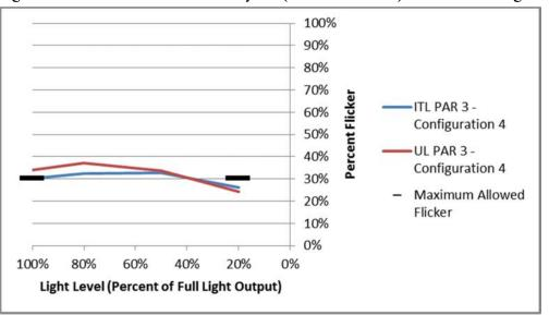
Figure 15: Round robin test results by lab (filtered <200 Hz) for PAR 3, configuration 4
