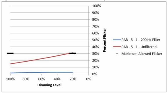
Figure 14: Filtered and unfiltered results for PAR 5, configuration 1
