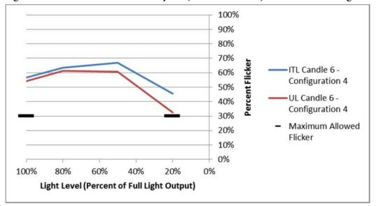
Figure 16: Round robin test results by lab (filtered <200 Hz) for Candle 6, configuration 4
