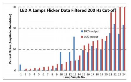
Figure 3: Filtered Flicker Test Data for 25 LED A-lamps (filtered flicker proposed for CA standards)
