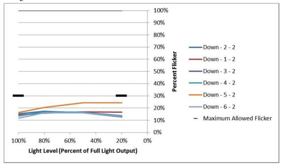
Figure 8: Percent Flicker (Filtered <200 Hz) vs. dimming level for all Downlights, configuration 2
