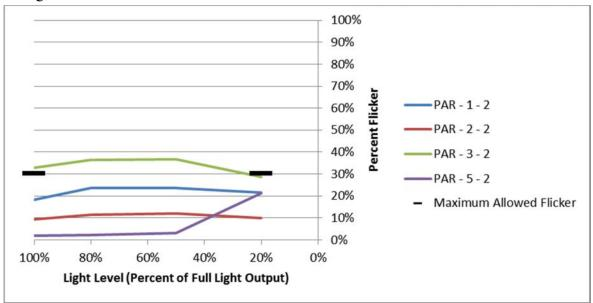
Figure 3: Percent Flicker (Filtered <200 Hz) vs. dimming level for all PAR lamps, configuration 2
