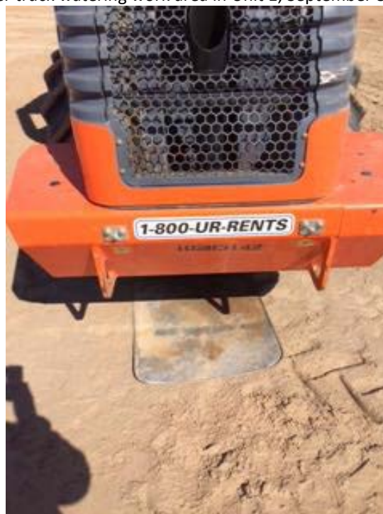
Photo 4: DF Bio-8: Minimize Spills of Hazardous Materials Drip pan used to negate contaminated soil in Unit 1; September 11, 2015
