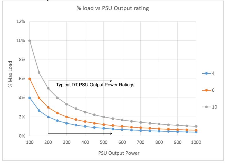
3 curves are 4, 6 and 10 watt idle load power Proposed Idle power limits forcing PSU operation below 6% rated load
