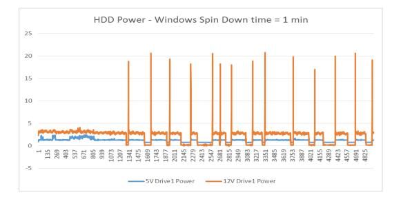
The test results provided in the figure above were collected on a Western Digital Blue 1TB hard drive with the hard drive spin down time set to one minute in Windows.
