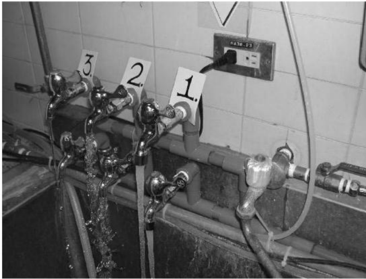
FIGURE. Experimental set up of the model plumbing system (1, faucets with aerators; 2, control faucets; 3, faucets with laminar water flow devices).
