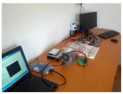
Figure 2. Complete setup for desktop power measurement
