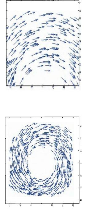
Quiver plots showing flux vectors near the receiver from a sample of heliostats for Option 1
