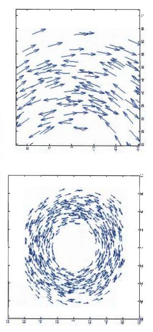
Quiver plots showing flux vectors near the receiver from a sample of heliostats for Option 2
