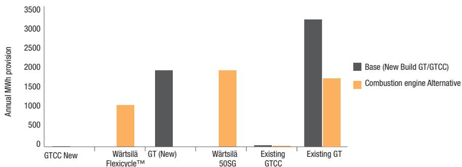
**Figure 5. Provision of Non-Spin ancillary service for the two scenarios. Due to fast start up times and high reliability, combustion engines provide 50% more Non-Spin than the gas turbine/Base buildout and reduce provision of Non-Spin by the existing GTs by 50%.**
