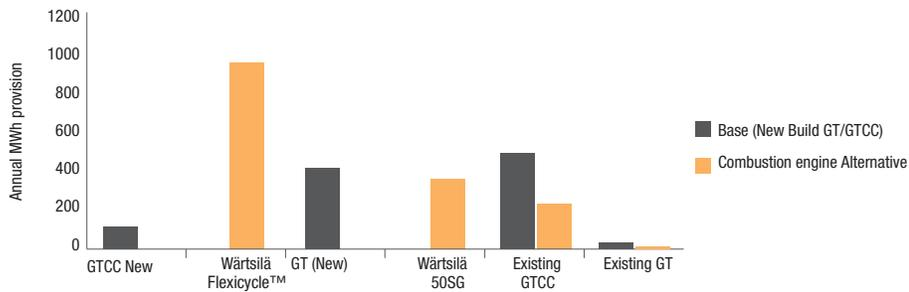
**Figure 3. Provision of Regulation Up (RegUp) ancillary service for the two scenarios. Combustion engines provide more than double the amount of RegUp compared to the gas turbine/Base buildout and reduce provision of this A/S by the existing GTs and GTCCs.**
