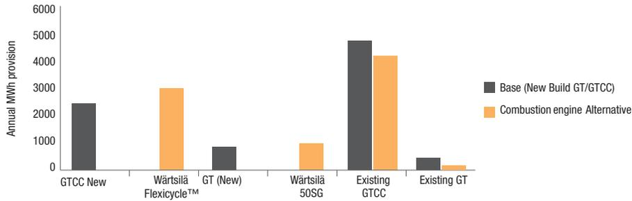
**Figure 2. Provision of Load Following Up (LFUP) ancillary service for the two scenarios. Combustion engines provide 30% more LFUP than the gas turbine/Base buildout, and reduce provision of LFUP by the existing GTs and GTCCs.**
