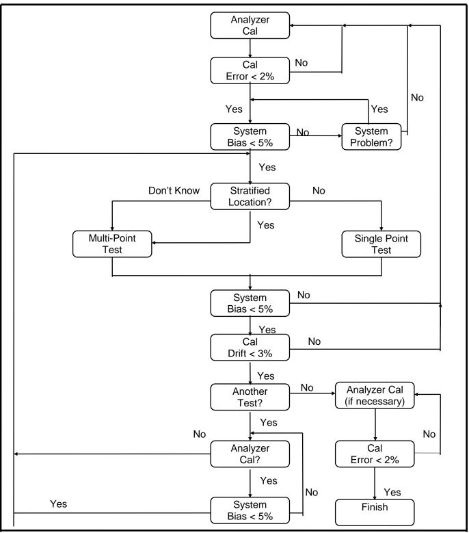
FIGURE 1: SDCAPCD METHOD 100 CALIBRATION AND TEST SEQUENCE
