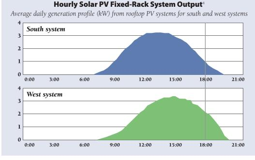
With time-varying rates, consumers will realize greater value from their PV investment by installing racking to orient the panels toward the west. Properly designed, this should compensate customers for any slight reduction of total PV output that results from this strategy – a significantly higher price per kWh for the same or slightly lower output.
