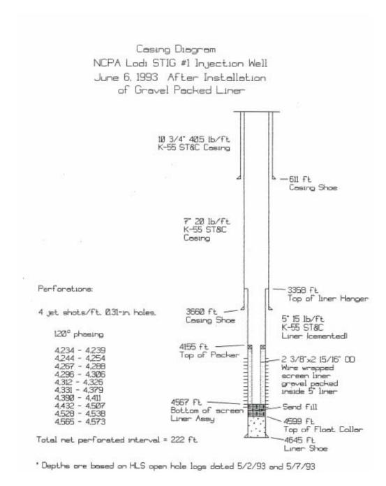
**Figure 2.** As-built constuction specifications for well STIG-1 (from Appendix 10 of the Permit Application).
