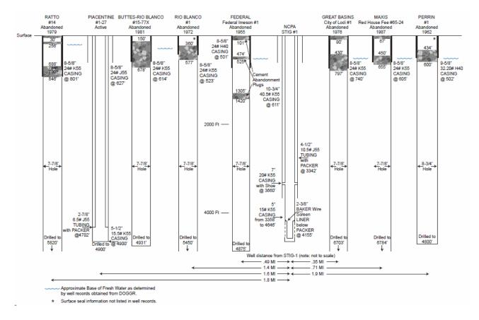
**Figure 3.** Wellbore schematics of the active and abandoned exploratory gas wells in the Area of Review.
