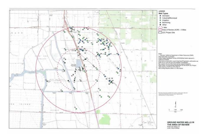
**Figure 4.** Map showing ground water wells within the two-mile Area of Review (from Attachment B of the Permit Application).
