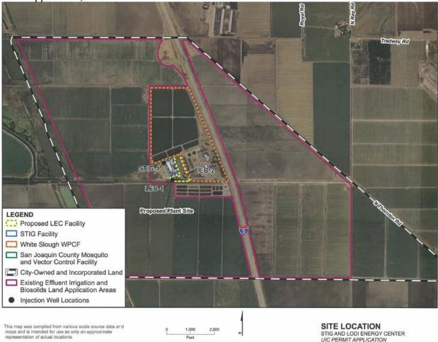
**Figure 2.** Site location of the STIG and Lodi Energy Center, showing the site of the proposed power plant, well STIG-1, and the proposed locations of wells LEC-1 and LEC-2 (from the Introduction to the Permit Application).
