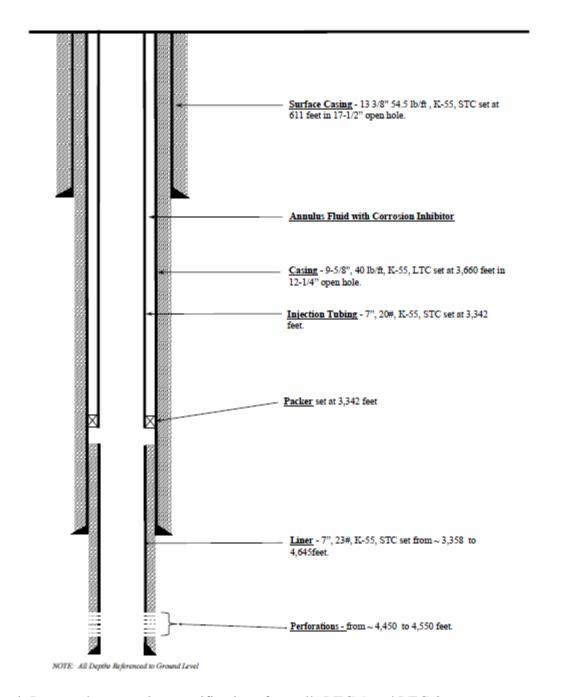
Figure 1. Proposed constuction specifications for wells LEC-1 and LEC-2.
