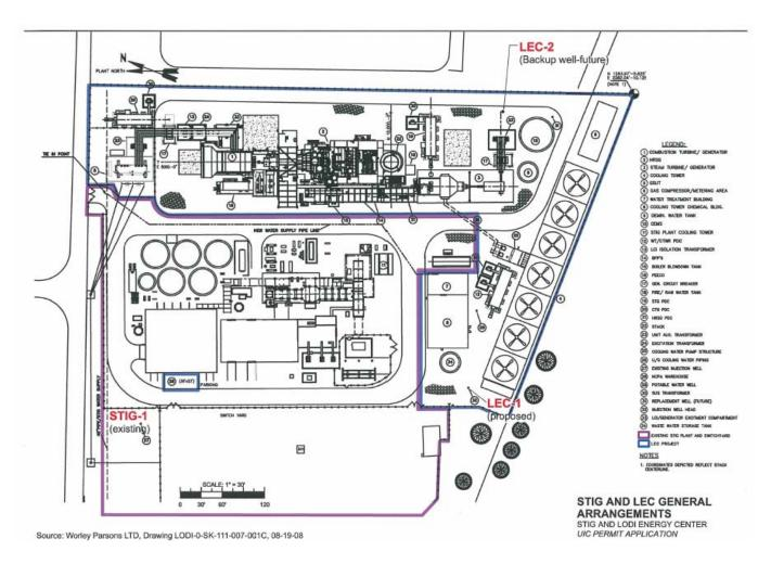
**Figure 3.** STIG and Lodi Energy Center general arrangements, showing the site of currently existing well STIG-1, and the proposed locations for wells LEC-1 and LEC-2 (from the Introduction to the Permit Application).
