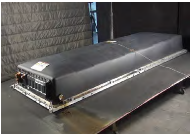
Figure 1-1: Example of UL 9540A Module Level Test [2]
