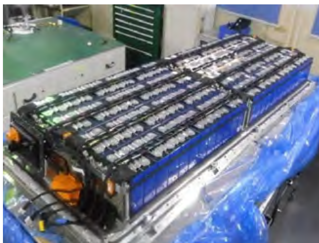
Figure 2-3: CATL Module containing 104 cells [2]
