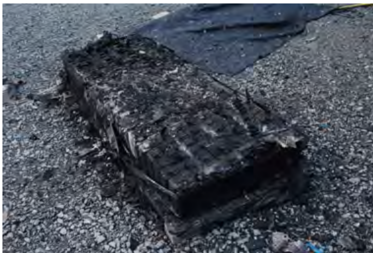
Figure 3-4 Module condition after pre-test
