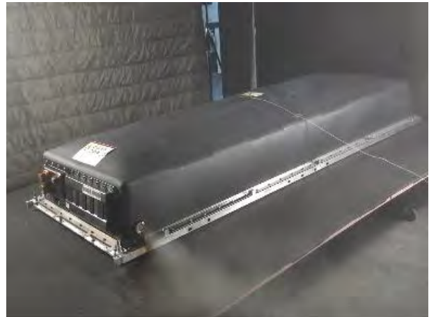
(f) Thermal runaway of adjacent cell 21-2 [01:07:12]
