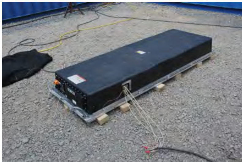
Figure 3-2 Module pre-test heater and control thermocouple wiring
