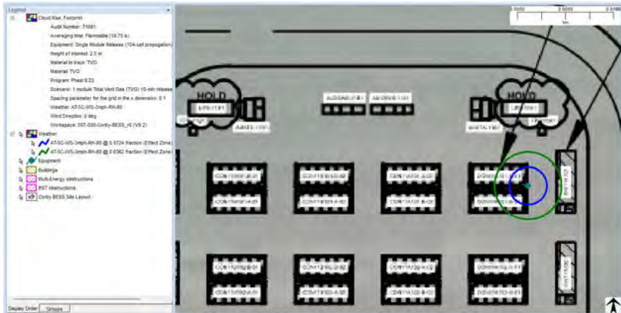
Figure 17. Map of horizontal extent of vapor cloud for LFL (7.24%) and 1/2 LFL (3.62%)
