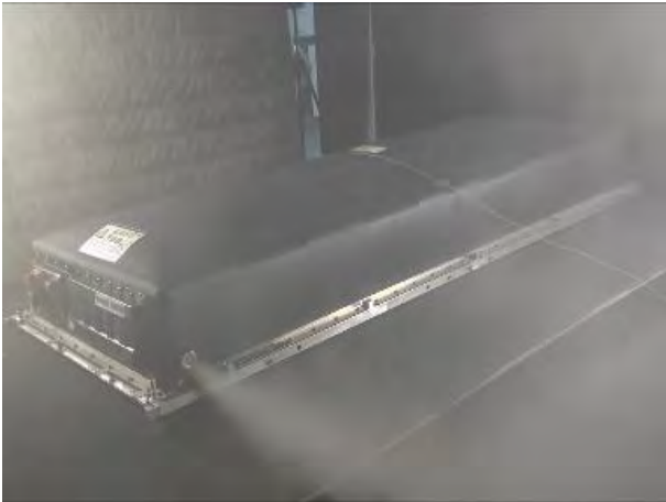
(e) Thermal runaway of adjacent cell 21-1 [00:54:54]
