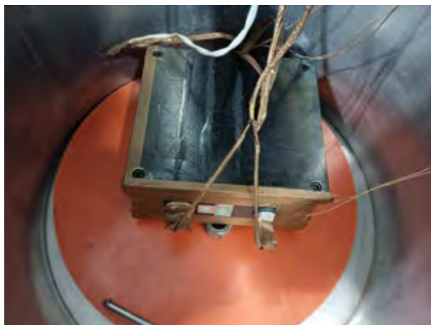
Figure 22: Sample 5 instrumented and inside gas test chamber
