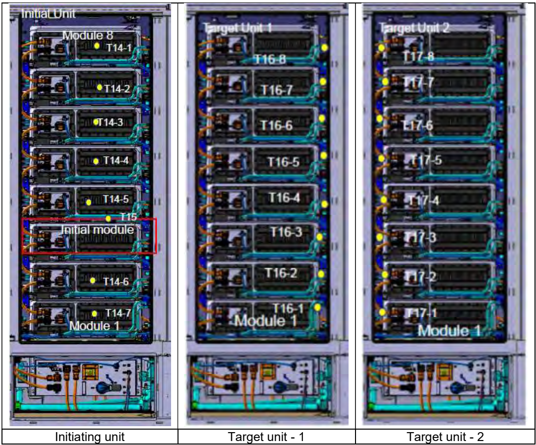
Figure 12: TC location in the initiating and target units, T16 series for target unit-1, T17 series for target unit-2
