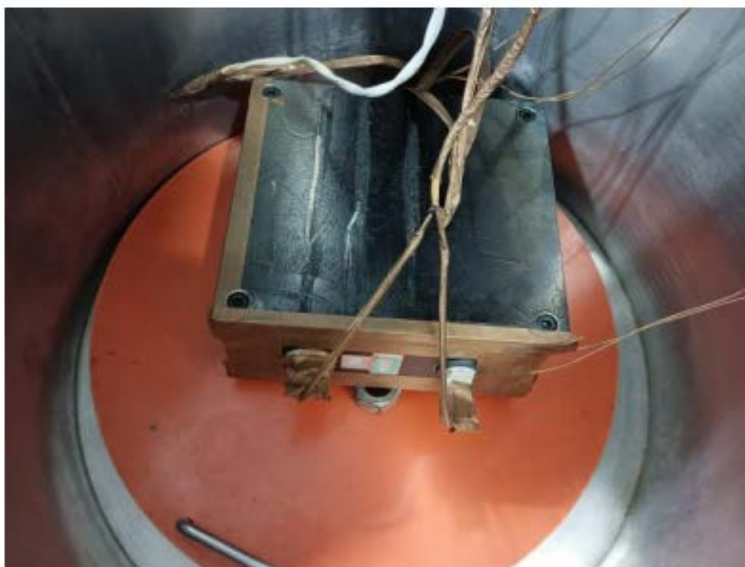
Figure 11. Sample 5 Instrumented Inside the Gas Test Chamber
