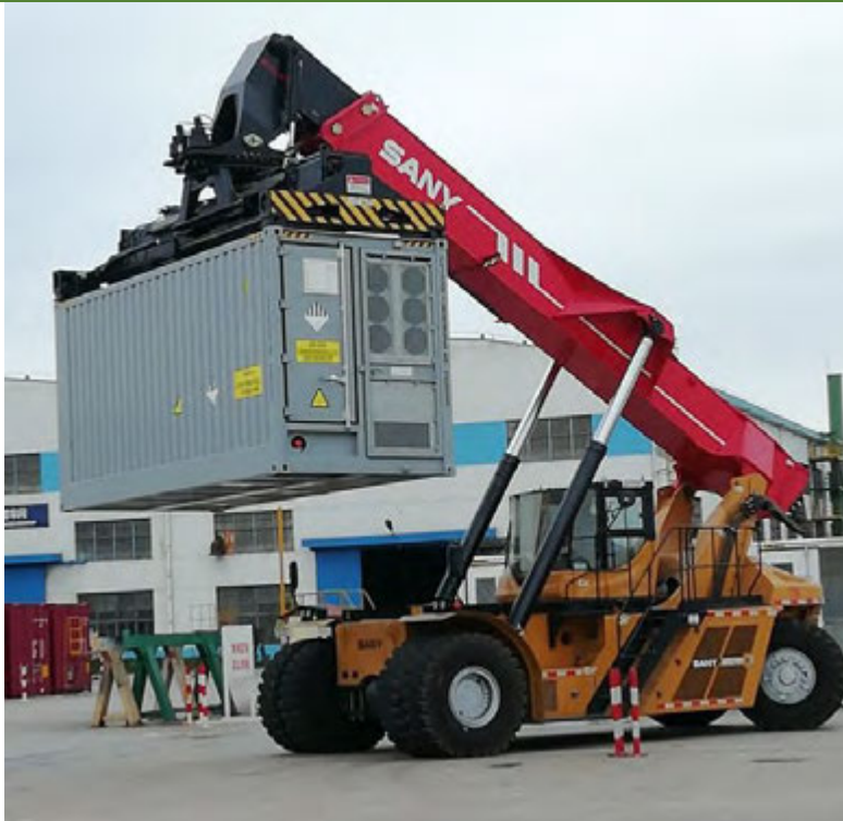
Figure 4-3 Top lifting by four points vertical crane
