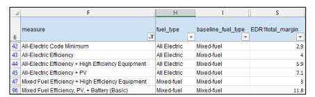
Figure 2. Single Family (625 square foot prototype) source energy margin results
