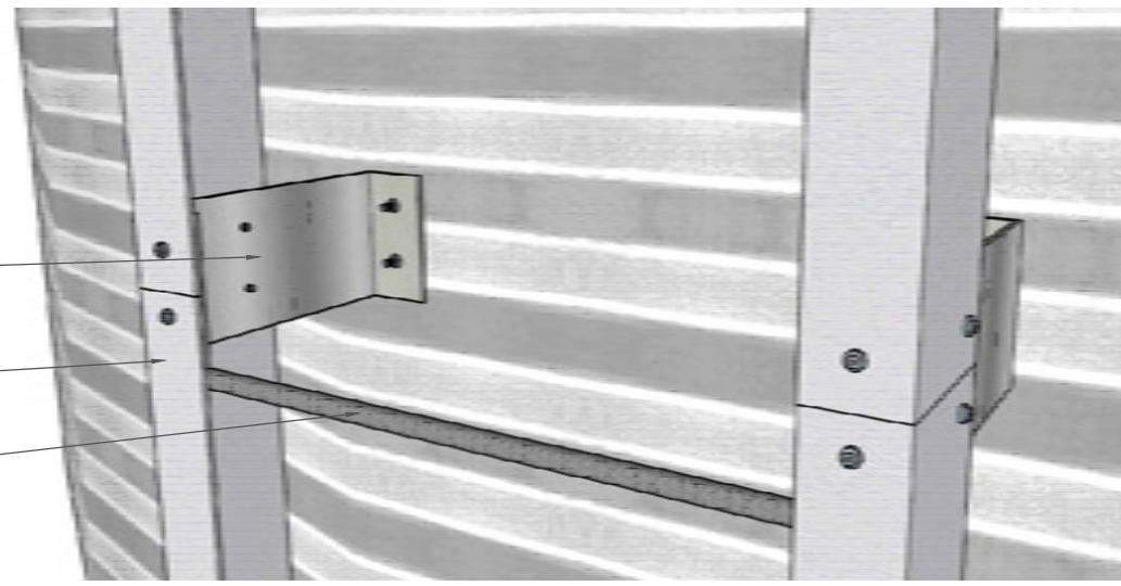
3-D VISUALIZATION OFF LADDER CONNECTION TO TANK WALL
