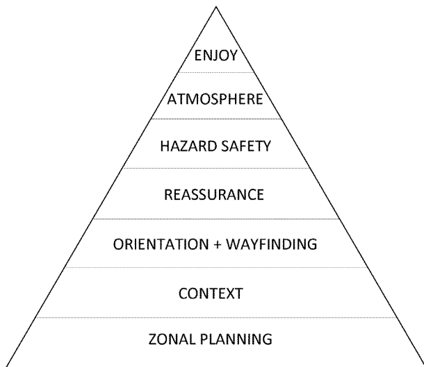
Figure 4-1. Hierarchical process of designing quality lighting for people in outdoor environments. The hierarchy begins at the largest wedge of the triangle, so planning lighting appropriate for the lighting zone is primary. Then, providing cues for the pedestrian of important destinations (hierarchy) and information on surroundings (context) is next. And so on. (Figure courtesy of Landscape Forms)
