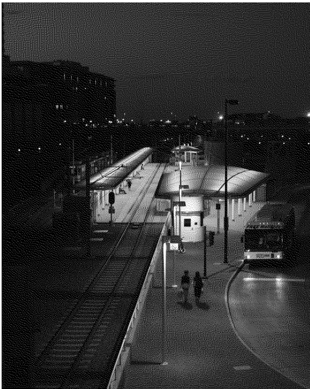
Figure 4-11. Fully shielded luminaires in an LZ-3 area provide a controlled glow confined within the train station. (Image courtesy of Clanton & Associates, Inc.)
