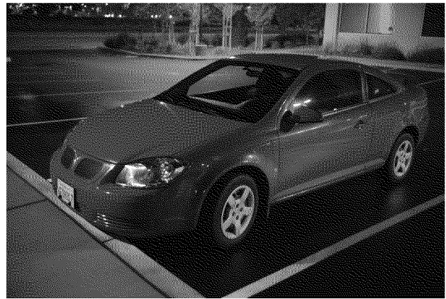
Figure 3-6. The effect of limited spectrum on a red car. The side is illuminated by low pressure sodium and the front by fluorescent store-front spill light.
