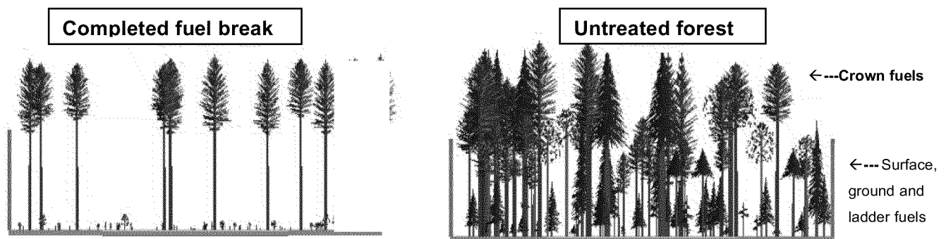
Figure 2. (Right) A typical fuel stratum for forest stands in California prior to fuel break installation. Fire behavior is a function of various inter-related elements including density of tree crown vegetation, smaller tree and brush “ladder” fuels, and ground surface vegetative debris. (Left) A completed fuel break
