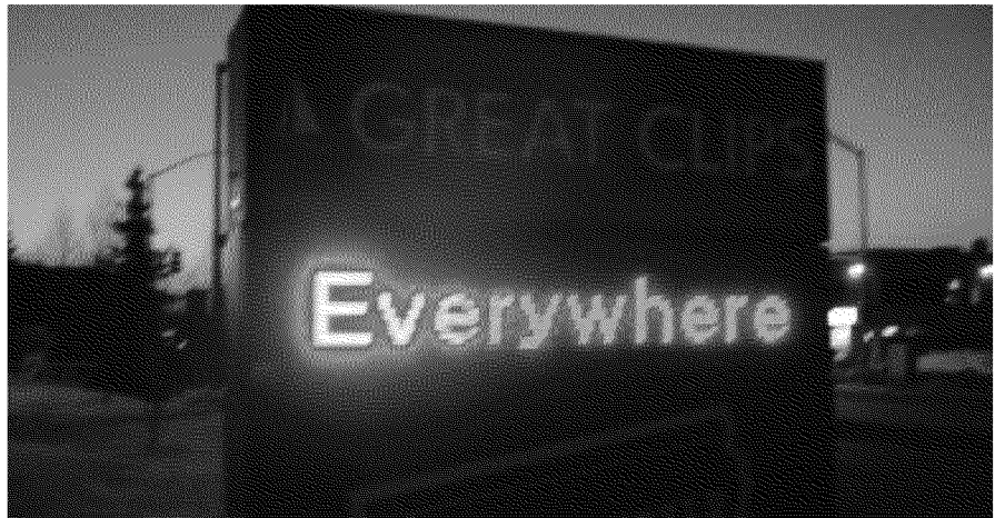
Figure 4-10. Excessive sign brightness a block away from an internally lighted sign. (Images courtesy of Clanton & Associates, Inc.)
