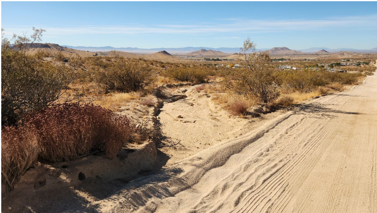
Photo Drainage 64a-1. Looking south at the eastern upstream end of Drainage 64a from the south side of Dawn Road. Flow direction from east to west. Soil scouring can be seen along banks.
