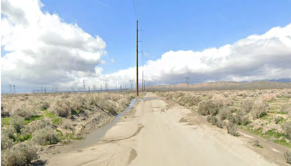
Photo 24. Looking west at Drainages 6 and 7. Photo was taken following a rain event to show run-off flowing down Rosamond Boulevard from Drainage 6 to Drainage 7, the result of clearing sediment from the road and redirecting flows.
