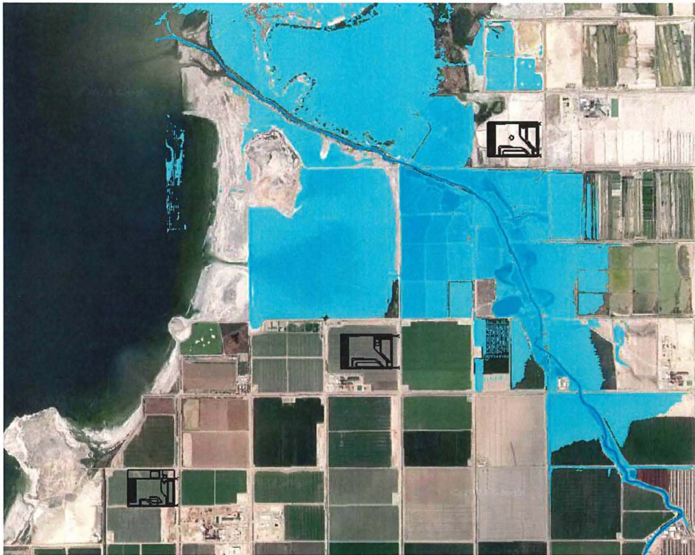
Figure 14. Alamo River Q100 floodplain under proposed conditions
