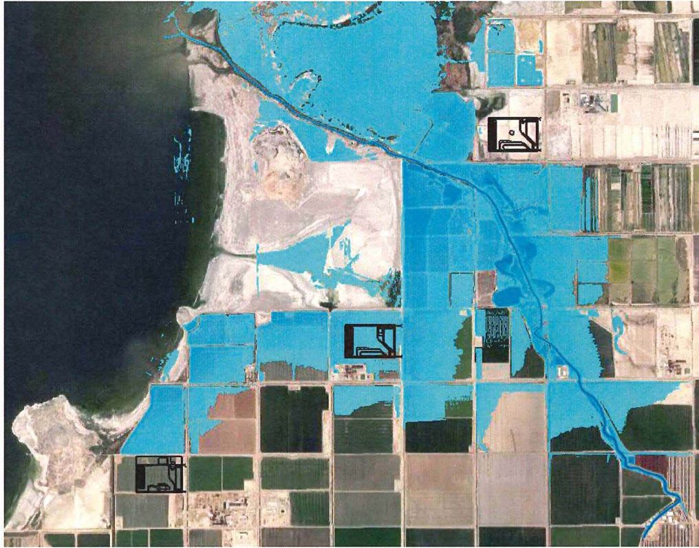
Figure 10. Alamo River Q100 floodplain under existing conditions
