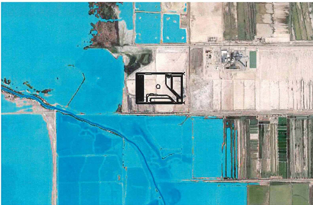
Figure 6. Morton Bay 100YR Flooded Area (identical under existing and proposed conditions)
