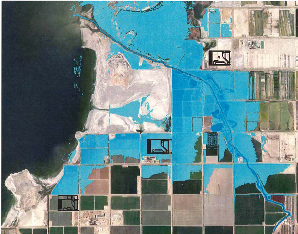
Figure 5. Alamo River Q100 floodplain showing the Morton Bay, Elmore North, and Black Rock locations. Additional details of the existing conditions for each of the project locations are included in the proposed conditions to allow for a direct comparison with the proposed conditions.
