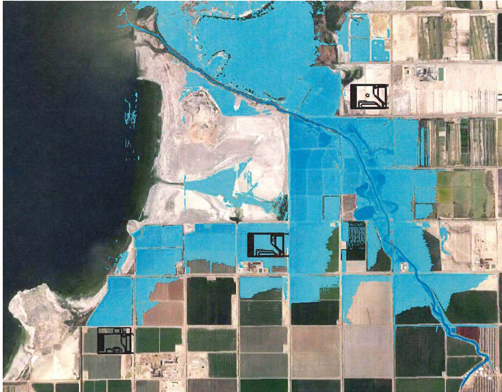
Figure 10. Alamo River Q100 floodplain under existing conditions
