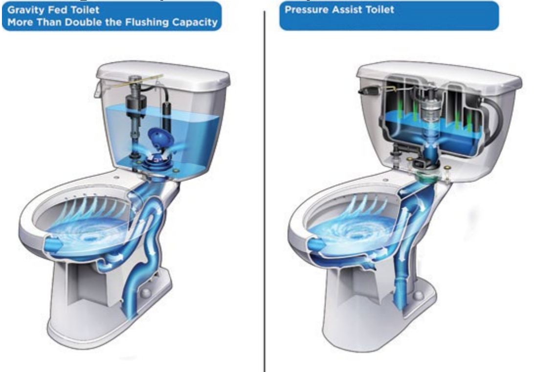
Figure 3-13: Diagram Comparison of a Gravity-Flush and Pressure-Assisted Toilet
