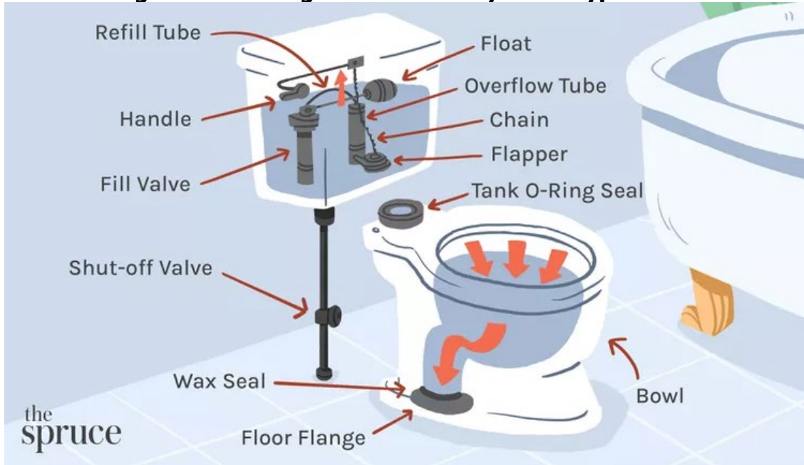
Figure 3-12: Diagram of a Gravity Tank-Type Toilet
