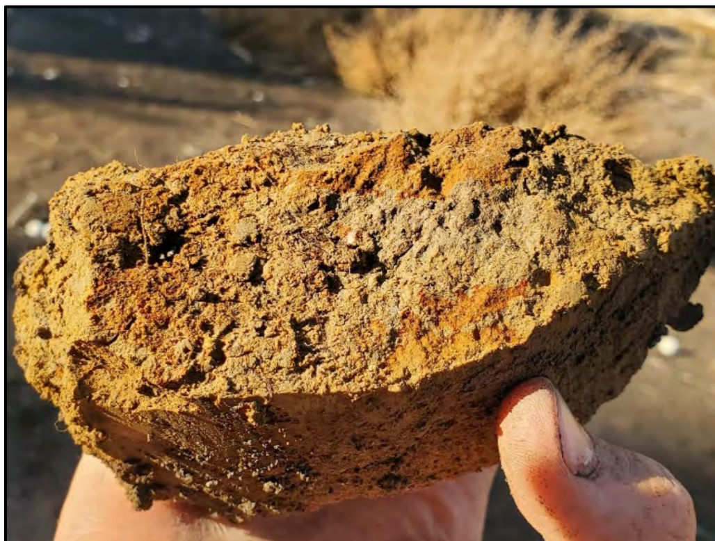
Photo 4. Representative wetland soil at data point 17 showing prominent redox features.
