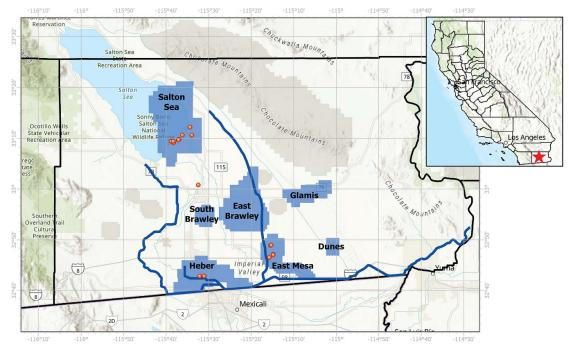
**Figure 1.** Map of the KGRAs (blue areas), geothermal power plants (red dots), Colorado River (dashed light blue line), and the major water canals (solid blue lines) located in Imperial County, California with inset showing the location of Imperial County in California shown with a red star.
