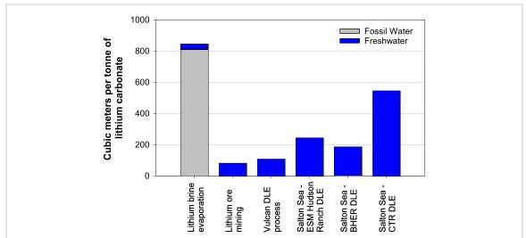
**Figure 3.** Water usage for different lithium extraction methods [32, 33, 37, 38]. DLE is direct lithium extraction. ESM is Energy Source Materials. BHER is Berkshire Hathaway Energy Renewables. (*Source*: adapted from Dobson *et al* [2] to include new data from Controlled Thermal Resources (CTR) [33]. Personal communication with CTR indicates this may overestimate water use but this has not been verified). Adapted from [2]. CC BY 4.0.
