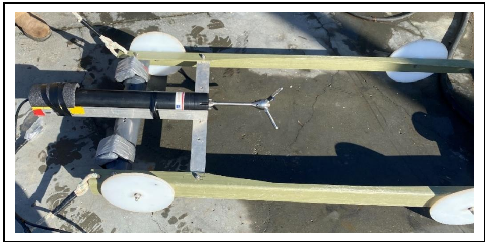
Figure 2-3. Sled-mounted Nortek Vector ADV.
